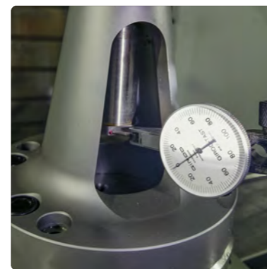
侧面开口处打表校正零件基准边 Calibrate the reference edge of the part at the side opening
