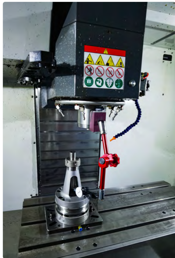
托盘在卡盘上快速装夹定位 Quick clamping and positioning of pallet on chuck
