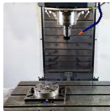
托盘在卡盘上快速装夹定位 Quick clamping and positioning of pallet on chuck
